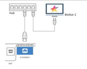
CoreStation has automatic MDI/MDI-X function, so it can be connected to a PC directly using a normal type CAT-5e cable.
