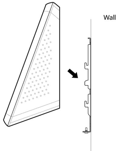
**4** Connect FaceLite to the bracket by rotating the product fixing screw of FaceLite.
