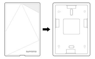
4 Assemble Xpass S2 with the extension bracket by screwing the mounting screws on the bottom of Xpass S2.
