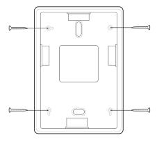
2 Mount the assembled extension bracket onto the desired place with the mounting screws for the bracket.
