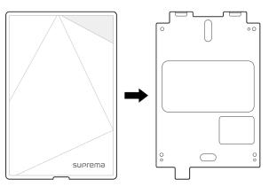
**3** Assemble Xpass S2 with the main bracket by screwing the mounting screws on the bottom of Xpass S2.
