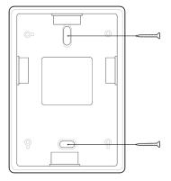
3 Attach Xpass S2 onto the mounted extension bracket.
