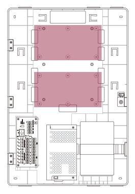
**2** After positioning the Input Module in the enclosure, fix it with the fixing screws.
