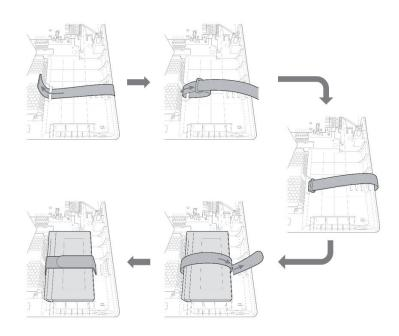
• Use a backup battery with 12 VDC and 7 Ah or higher. This product was tested with 'ES7-12' battery of 'ROCKET'. It is recommended to use a battery corresponding to 'ES7-12'.
