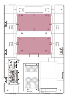
**2** After positioning the Output Module in the enclosure, fix it with the fixing screws.
