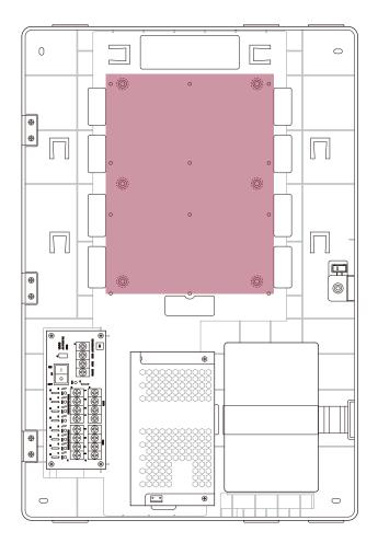
**2** After positioning CoreStation in the enclosure, fix it with the fixing screws.
